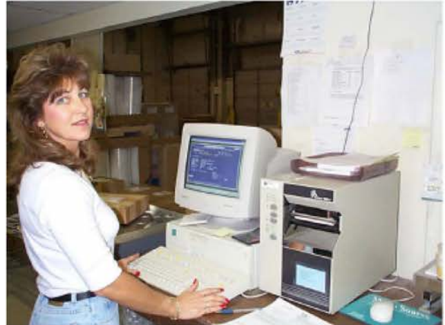
Computerized Shipping System: including electronic scale, PC and bar code label printer.
